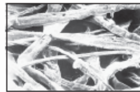
When all mechanisms are combined and utilized by a deep bed of the correct type of filter material, removal of virtually all particles whether liquid
