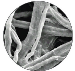
Cellulose fiber at X500 magnification
