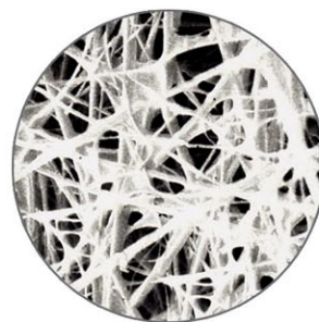
Micro-glass fiber at X500 magnification
